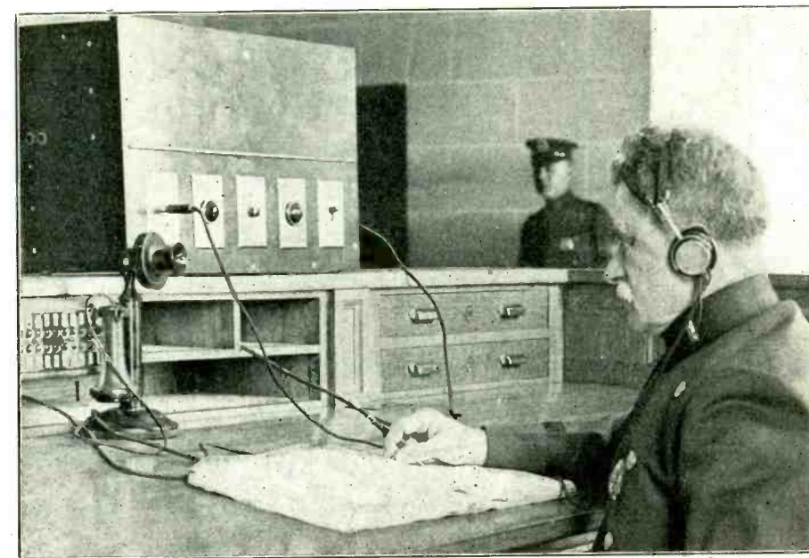
THE NEW POLICE RADIO ALARM—To left and right of the center plug are the signal lights. These are actuated from Police Headquarters. The light may be flashed at a single station, at several stations or at all stations at once. It means: "Listen in! An important police warning will be broadcast!" The device was demonstrated at the Police Conference. (Fotograms.)
